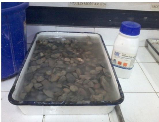
Figure 2. Treatment of RCA with sodium metasilicate.
