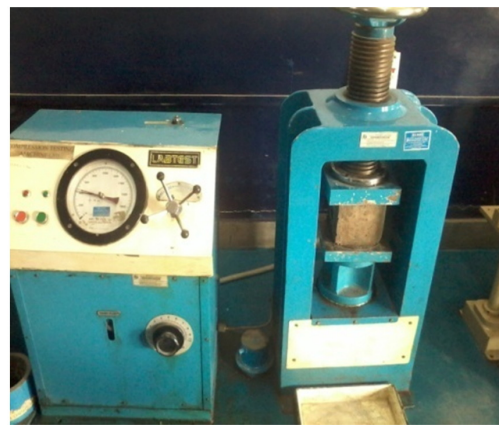
Figure 3. Testing of sample using CTM.
