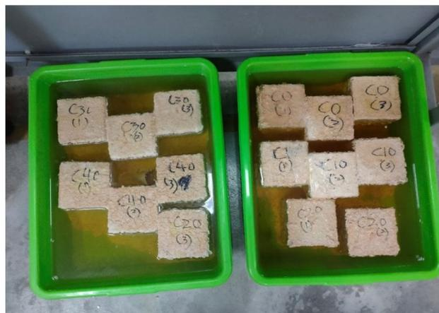
**Figure 4.** Immersion of concretes in 5% sulphuric acid solution.
