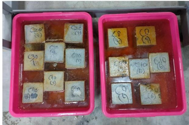
**Figure 3.** Immersion of concretes in 5% hydrochloric acid solution.
